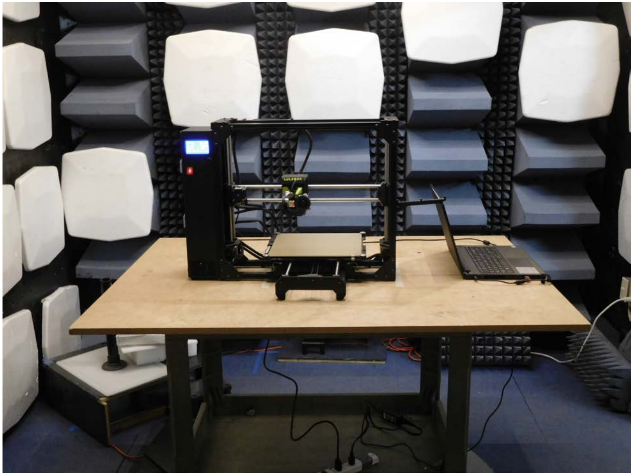
Test setup for Radiated Emissions - usb
