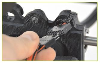
Evolution of the four locking connectors on the back of the electronics case enclosure. Each connector matches a keyed plug, which may require rotating the plug until the keys line up and the plug can be pushed in. Once the plug is pushed in, turn the locking sleeve clockwise until it is tight against the electronics enclosure.
