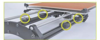
With the print surface facing up and the stepper motor end of the Y axis facing back, slide the Y axis assembly on to the Y axis mount brackets, aligning the holes on the brackets with the bolt holes on the Y axis assembly.
