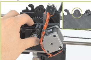
Plug in the tool head. Note the pin orientation:
