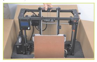
Carefully remove the entire printer frame from the box and set it on a sturdy, flat surface near an electrical outlet. Now you are ready to set up your LulzBot™ TAZ 3D printer!
