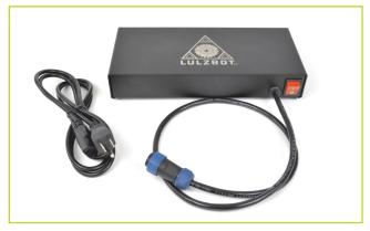
Locate the blue 24VDC output cable plug from the power supply. Connect the blue power supply plug into the keyed power supply connector on the printer electronics enclosure. Once the plug is pushed in completely, turn the locking sleeve clockwise until it is tight against the electronics enclosure. Hand tighten only!
