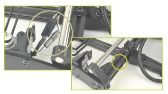
With the included 2.5mm hex driver, locate and remove the 3mm tool head screw in the top center of the X axis carriage. Next, take the tool head out of the Accessory Tray foam insert.
