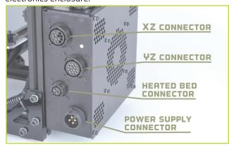
large straight plug from the XZ cable. The next connector down matches the large angled plug from the YZ cable. The third connector matches the smallest plug, from the heated bed cable.
