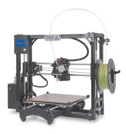
Remove the print bed assembly (Y axis) packed in the body of the printer by sliding it up approximately 15 cm (6 inches), freeing it from the black packing foam.
