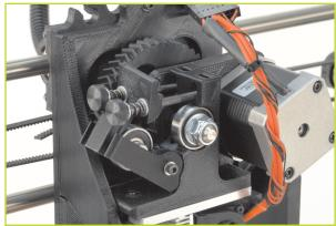
■ Once the filament extrudes a small amount out of the nozzle, raise the idler and slide the two idler bolts and plate back into place. Tighten the two idler bolts. Tighten the two screws until the top of the thumbscrews are about 10-11mm away from the plastic clip.
