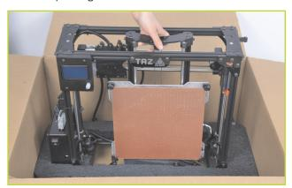
**B** Rotate the print bed assembly (Y axis), tilting the bottom toward front of box. Lower the print bed assembly (Y axis) into the box so it is parallel with printer frame, then it lift out and set it aside.
