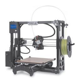
A Remove the printer bed assembly (Y-axis) packed in the body of the printer by sliding it up 6", freeing it from the packing foam.
