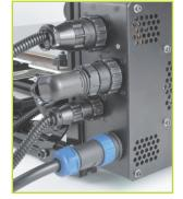
1 2 Plug the AC power cable into the power supply. Then plug the other end into an AC power outlet.
