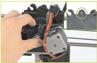
Plug in the tool head. Note the pin orientation— The tool head connector should have a small gap in the pins on the right hand side. When fully seated the connectors should fit flush against each other.
