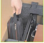
While keeping the printer in the box, pick up by the black aluminum frame and rotate the printer and foam 90 degrees - setting it upright within the box. Make sure name plate at top is UP. Remove top foam.
