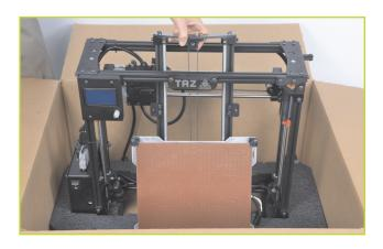
**C** Carefully remove printer frame from box and set it on a sturdy, flat surface - you're ready for assembly!
