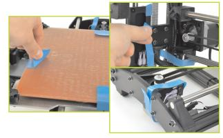
Locate the four Y axis bolts on the TAZ frame (see green circles below). Turning counter clockwise, remove each Y axis bolt and set aside.
