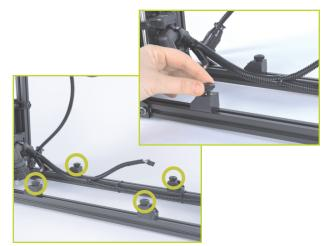
**3** Locate the four Y axis mount brackets on the TAZ Y axis.
