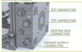
straight plug from the XZ cable. The next connector down matches the large angled plug from the YZ cable. The third connector matches the smallest plug, from the heated bed cable.
