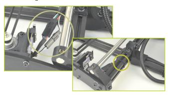
6 Locate and remove, with the included 2.5mm hex driver, the tool head 3mm screw in top center of the X axis carriage. Remove the extruder head from the Accessory Tray foam insert.
