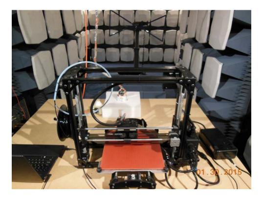
Radiated immunity test setup - 80-1,000 MHz
