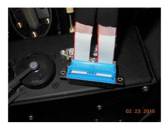
A blue LCD cable connector was used during emissions testing, changing from a more expensive version of the same connector. The results were the same or better using the less expensive connector.
