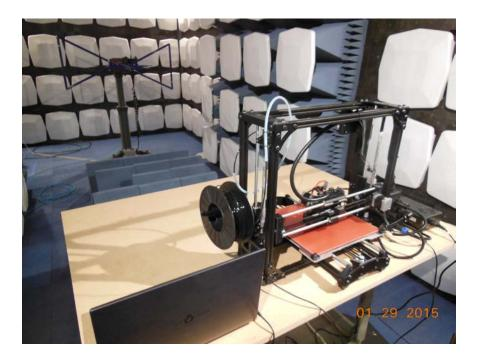
Radiated emissions test setup
