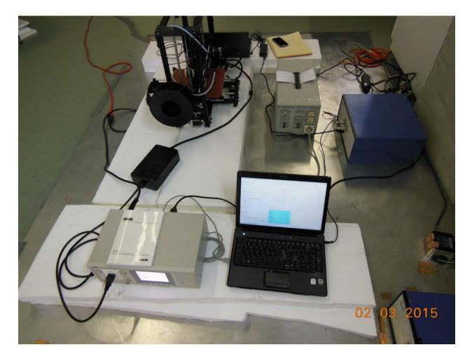
Test setup for AC power line harmonics
