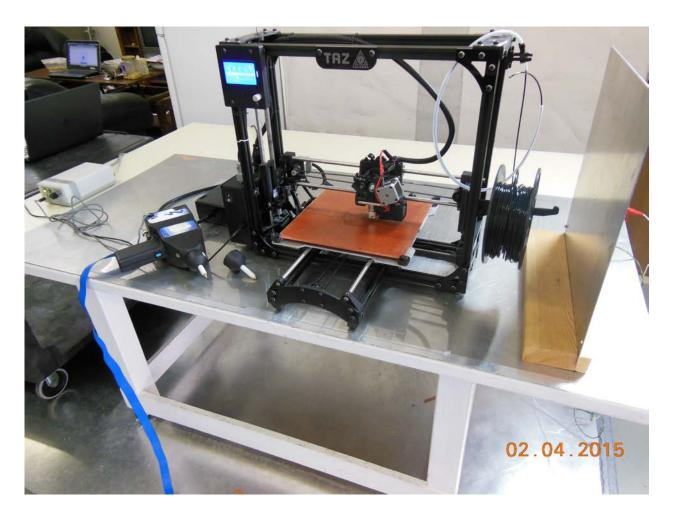
ESD test setup per EN 61000-4-2 Horizontal and Vertical coupling planes were checked
