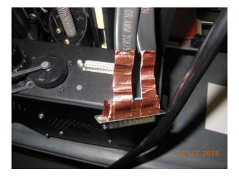
Copper tape was added to the ribbon cable shielding to connect the shield to the metal of the connector in order to get a chassis ground connection.
