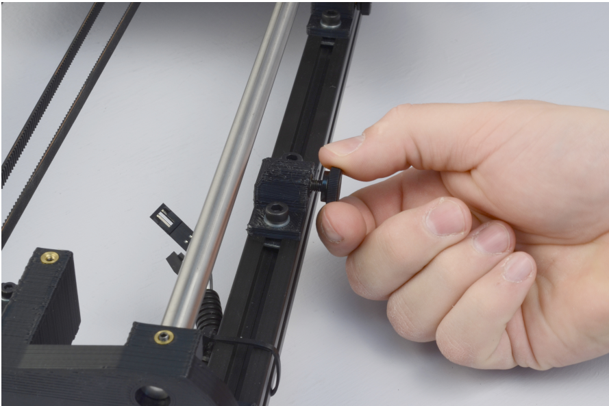
Figure 1.3: Remove the four Y axis bolts
