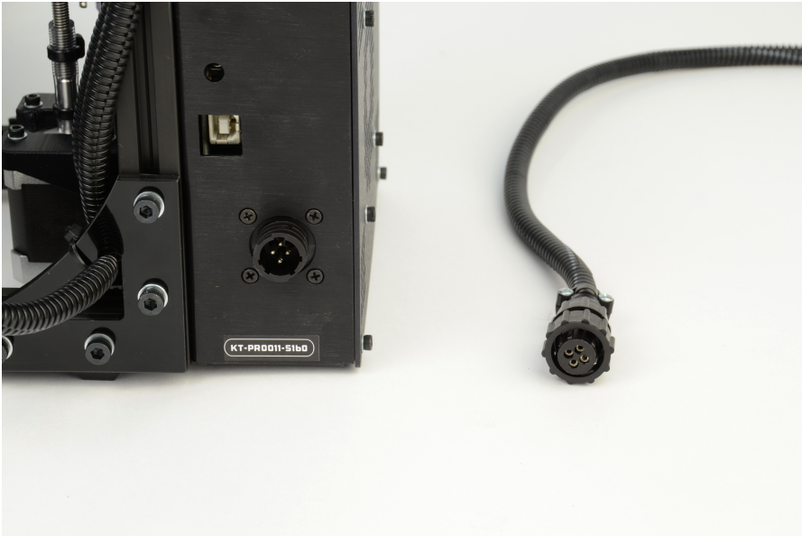
Figure 1.16: 12V DC Power supply plug and receptacle
